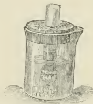
Beaker and tube for the dialysis of liquid poisons.
